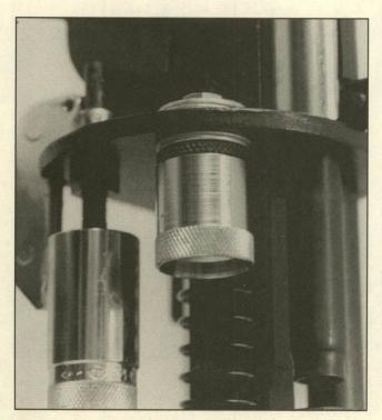
If your press is equipped with a non-adjustable crimp starter, placing washers between the die and tool head can effectively lower die position. The two washers above the crimp die have lowered the starter the needed amount. The two washers on top of the die plate are spares.
