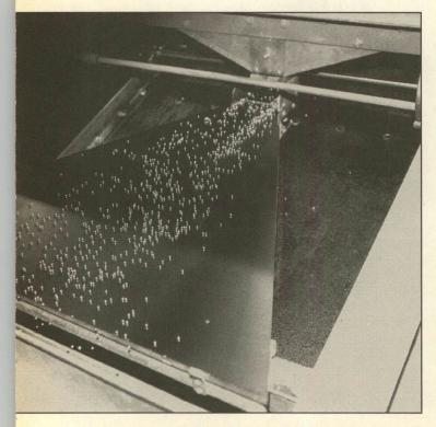
This is newly formed shot rolling down inclined plates which separate the less than perfectly formed pellets from the most round spheres.
