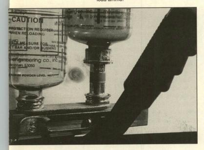
Powder measure baffles can increase the uniformity of metered powder charges.
