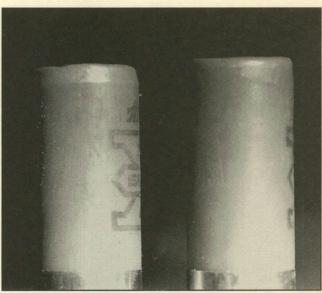
The case on the left has a heavy bevel on its mouth to provide smooth feeding and uniform ballistics compared to the case on the right which has no bevel.
