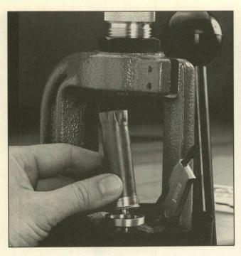
With all the shells to be reloaded properly decapped and sized, the die body must now be changed to a primer seating unit. Remove the top die bushing and decapping rod assembly. Drop the priming tube assembly into the die and replace the die bushing. Remove the standard shellholder and replace it with the priming cup. Remove the sizing ring to prevent cases from jamming in the die body during priming. The die is now ready for use.
