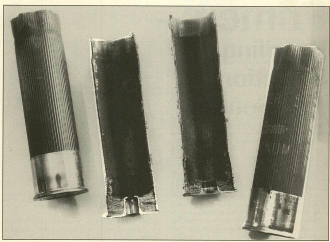
Cutting cases in half can help verify identification or illustrate that what appears the same on the outside is not necessarily the same internally. Note that both cases are external look-alikes, but the internal base wad configuration is noticeably different. The case on the left is a Riefenhauser type with a high inner base wad; the case on the right, a Riefenhauser with low inner base wad. These cases require substantially different reloading data.
