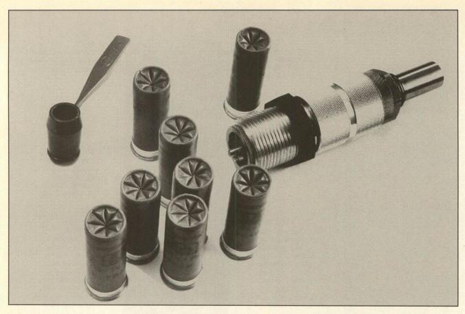
The reloader can assemble a box of shells in about an hour with a basic die set used on a metallic cartridge reloading press. The crimps shown are typical of the results you will obtain.
