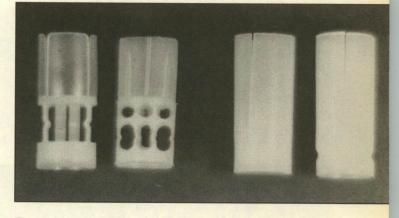
The wads on the left are lead shot wads (a Winchester AA type on the extreme left and a Remington Power Piston). Those on the right are two steel shot wads made of a thicker, tougher plastic and having no collapsible leg section.
