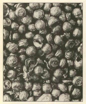
Not all homemade shot makers produced acceptable pellets. This mess was made on a unit that helped give home shot making a very bad name.
