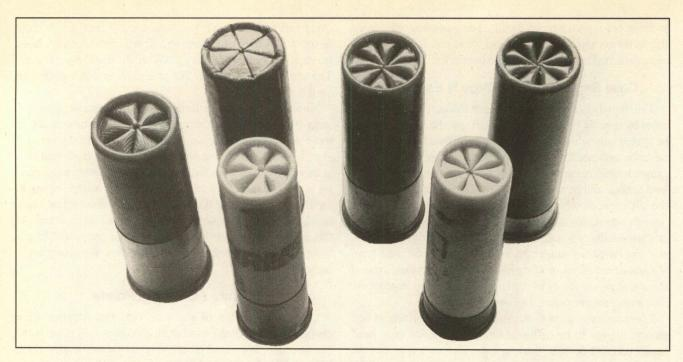
The number of folds (six or eight) in a case's crimp do not affect ballistics, though the appropriate crimp starter must be used when reloading.
