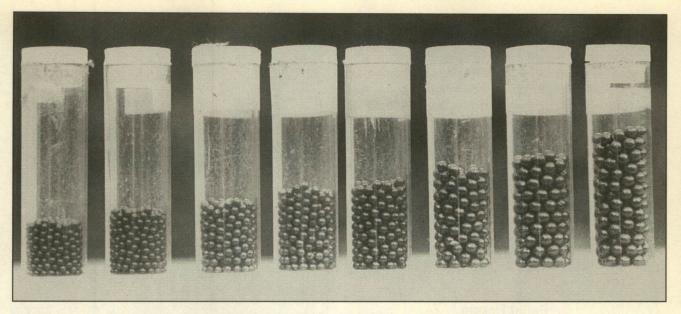
Shot comes in a number of sizes. As pellet size is increased, the shot charge weight must be increased to maintain sufficient pellet count for proper pattern density. Each of these containers have identical numbers of pellets which range in size from #9, through #81/2, #8, #71/2, #6, #5, #4, and #2.
