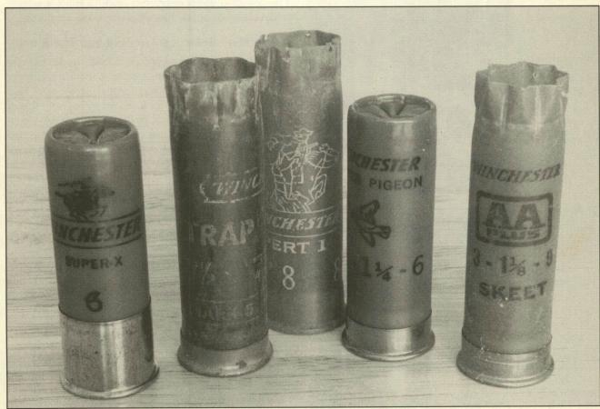
These 12-gauge 234-inch cases are all Winchester compression-formed hulls and use identical loading data.
