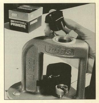
In order to load shotshell ammunition on a rifle/handgun reloading press, the press must have a removable  $1^{1}/_{4}$ " x 12 threaded bushing.
