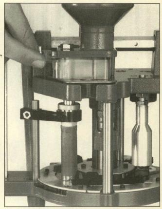
Pick up a wad with the right hand, and place it into the wad guide. Simultaneously place another shell into the first station of the tool with the left hand. Pull the press handle down using the right hand. This will seat the wad into position, deprime the case in station one and prime the case in station two. With the press handle down, meter the powder and shot levers and drop a new primer into the primer tube.
