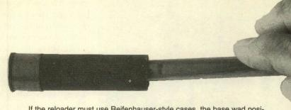
If the reloader must use Reifenhauser-style cases, the base wad position must be verified with a homemade marked dowel.
