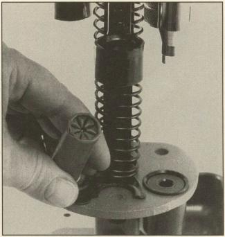
Another improper crimp die adjustment can cause a crimp set too deeply that fails to properly seal the shot in the case.
