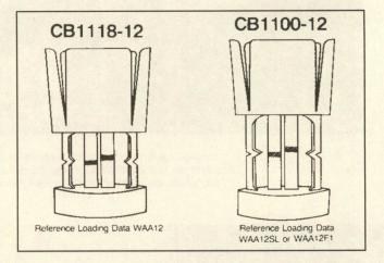
These wad designs, in straight-wall and tapered-wall styles from C&D Special Products, are available in 12-, 20-, 28-gauge and 410-bore for target loads..
