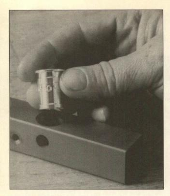
Install the correct powder and shot bushing for the load selected. Verify thrown charge weights with an accurate scale as bushings and bars will throw varying charges dependent upon a number of conditions. The actual charge thrown may be heavier or lighter than specified by the bushing manufacturer.
