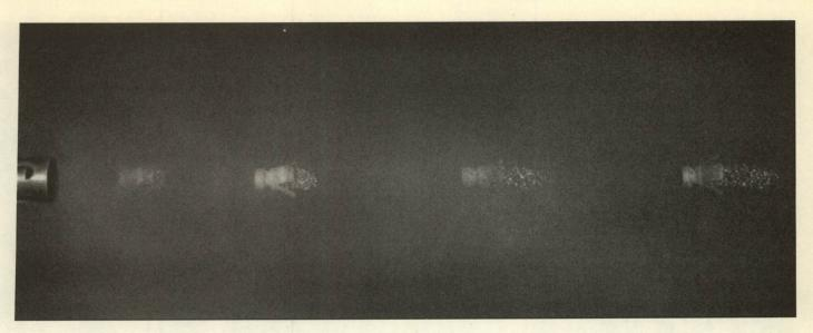
This is a Winchester charge of 11/8 ounces being propelled from a target load at 1200 feet per second. Note how quickly the AA wad opens and begins to fall away from the shot column.
