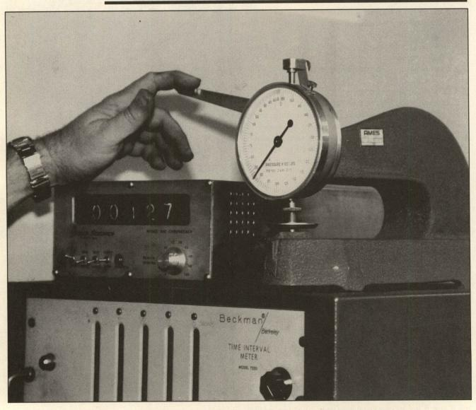
In the lead crusher testing system, the "crusher" length is properly measured with a bench-style gauge rather than a hand-held micrometer.
