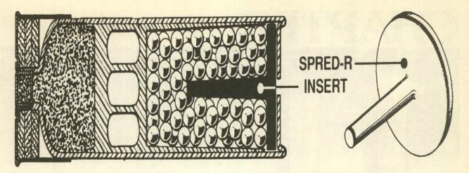
The Polywad Spred-R-Wad is a variation of the cardboard spreader. It's designed to open patterns from Full to Improved Cylinder and can be used with any wad and shot. Shaped like a thumbtack, it's inserted into the shot charge just before the crimp is applied.
