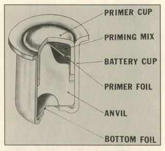
This is the typical construction of a shotshell primer. Although, some primer types do not have a bottom foil or seal to prevent fine grain spherical propellants from entering the primer.
