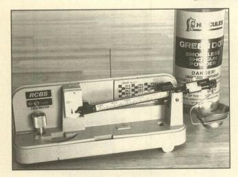
A powder/shot scale is a basic and essential tool for the assembly of safe shotshells. Shotshell reloaders will do best to purchase a scale with a 1000-grain capacity.
