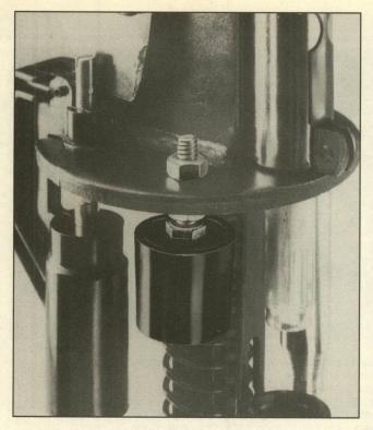
A good crimp start die, such as this Mec Spindex, rotates freely to align precisely with the original crimp. It is also adjustable up and down for the correct amount of preclosing.
