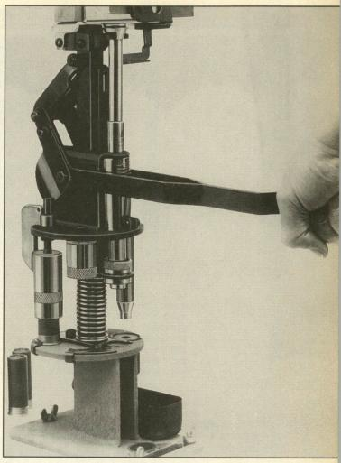
The final crimp die must be adjusted to give a crimp as close as possible to the original factory load. It should also be capable of putting a good bevel on the loaded case mouth. The die shown has all the necessary adjustments.
