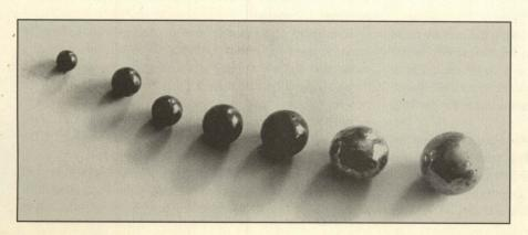
Shot sizes being loaded will have a direct bearing on the metered charge weight of the pellets. The smallest shot sizes will result in the heaviest charges and the largest sizes in the lightest charges (see text).
