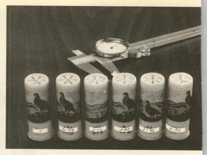
A good dial indicating caliper is essential for duplicating the overall shell length and depth of crimp of factory loaded shells. Overly short or long measurements can drastically alter ballistics.
