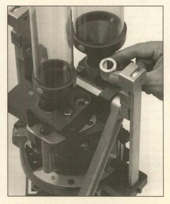
Install the appropriate powder and shot bushings in the press. Actual metered charges must be verified prior to reloading.
