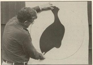
Placing a life-size silhouette over the test patterns can help in evaluating a load and choke combination. An acceptable average pattern will not have pellet-free patches large enough for a silhouette to fit inside with fewer than five shot pellets in the targets' vital area. In the case of the turkey being used here, it would escape multiple head and neck hits.
