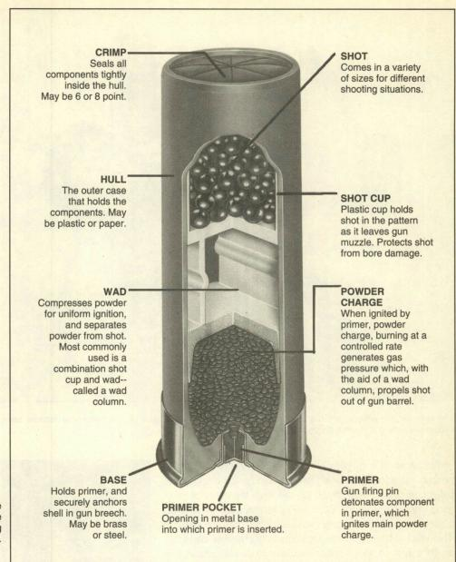
This cutaway shell shows the various components the reloader will replace during ammunition assembly.
