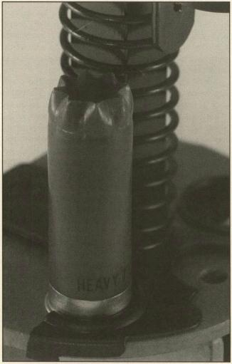
A good crimp begins with a proper crimp start. Shown is a typical eight-point crimp start. The case should display well-formed petals and be 25 to 35 percent closed.
