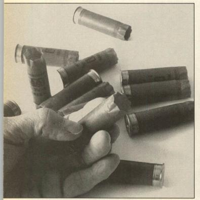
Inspect each case for its suitability for reuse and carefully segregate cases by types.
