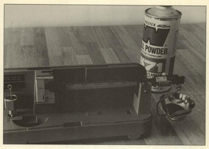
The charges metered by powder and shot bushings and bars can vary greatly from what may be an expected weight. Metered charges must always be verified with a powder and shot scale under exacting conditions.
