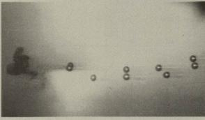
At 6 feet from muzzle minimum dispersion of pellets and superior sphericity are apparent.
