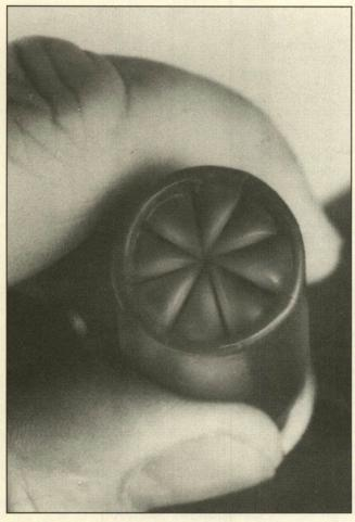
Finally, slide the shell into position under the final crimp die, using the left hand. Pull the press handle all of the way down and then up with the right hand. Remove the fully loaded case from the reloading machine. The crimp should look very similar in shape and depth to a factory load. If it does not, the crimping die needs adjustment. Follow the press manufacturer's instructions to do so. Also read Chapter 11: Crimps and Ballistics.
