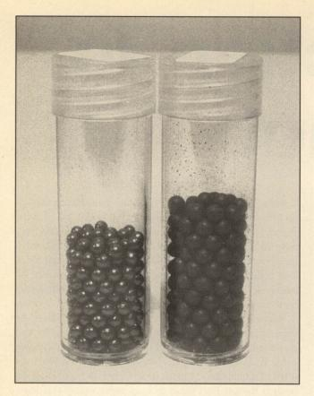
Here are two containers comparing lead versus steel pellet density. The one on the left contains 13/8 ounces of lead #4 pellets. The one on the right contains a lighter charge of 11/4 ounces of steel #2 pellets. If density alone was not enough of a problem, steel requires the selection of pellets about two to three sizes larger to maintain downrange ballistics and penetration.
