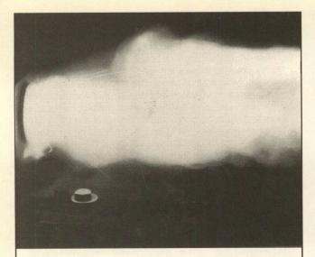
Shotshell component primer. Flash photograph (70°F). Note the large volume of white-hot gas being discharged.
