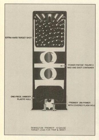
Shotshell ballistics are built into the case. The type and quantity of components used, as well as case construction will determine the ballistic performance of the shell. The actual shotgun used will have little bearing on the load's performance.
