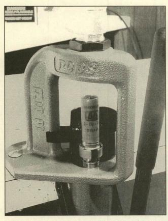
The final crimp removes any slight riveting of the case mouth (which could cause feeding malfunctions and chambering difficulty) and puts a bevel on the crimp area to help firm it up. RCBS suggests this as an optional step, but we feel it is essential for top ammunition performance.
