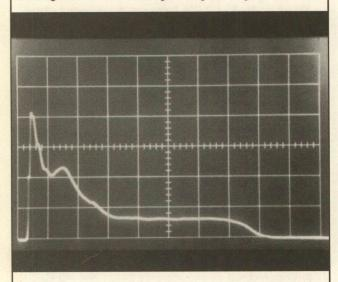
Shotshell component primer. Intensity of energy being released (70°F). Graph measures intensity vs. time in milliseconds.
