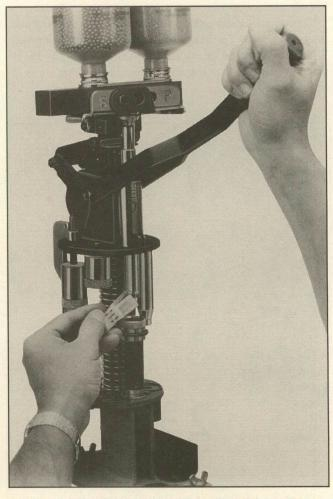
The wad plays an important role in the ballistics obtained and the uniformity of those ballistics. The reloader must select wisely and use only the specific wad listed in the data source.
