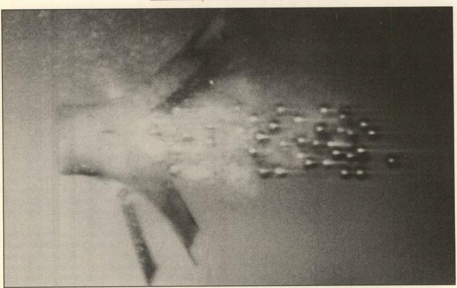
The largest pellets at the highest velocity will travel the greatest distance. Safety demands the shooter be familiar with the maximum range of the pellet/velocity combination being shot. This is a charge of #2 pellets as delivered from a Federal 10-gauge Premium load.
