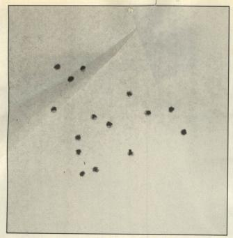
This pattern of 00 buckshot covers less than an 8-inch diameter at 20 yards. The same load at 25 yards would stay under the 15-inch maximum allowable buckshot pattern diameter.
