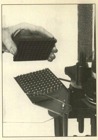
Automatic primer feeds can speed up the loading operation. However, when primers are placed into bulk storage (as they would be in the auto feed magazine) they represent a potential risk with respect to spontaneous ignition. Auto primer feeds are best used by an experienced reloader who has learned the caution required.
