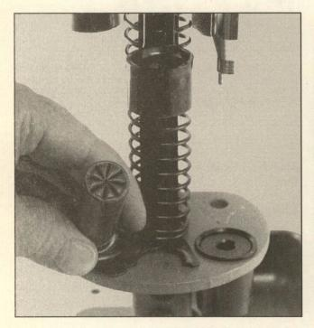
A common mistake is to form a shallow crimp which can later open up.
