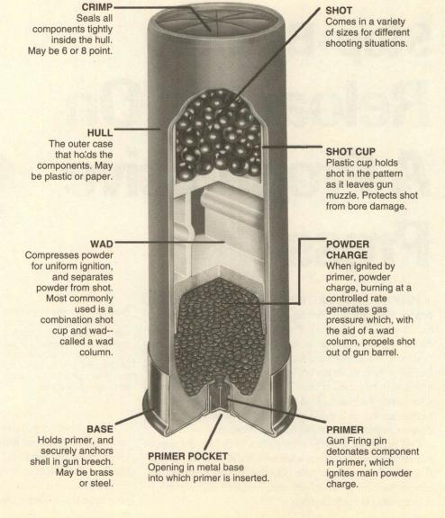
Properly inspect and segregate fired cases prior to reloading.
