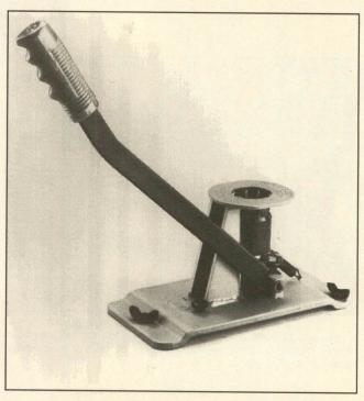
Remote sizing units are necessary when using progressive tools that do not supply a sizing die as part of the basic setup or that do not allow for heavy-duty sizing (over-expanded cases or high metal head cases).
