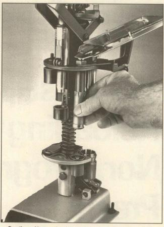
Caution: Always check to make sure there is no foreign material in the primer station before placing the primer into it. If a loose pellet or other material falls into the primer station, the primer could be ignited during seating and present a hazard to the reloader.
