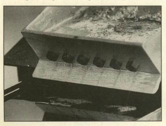
This is a close-up of the lead droplets escaping from a Littleton shot maker and falling into the oil bath to harden the pellets.
