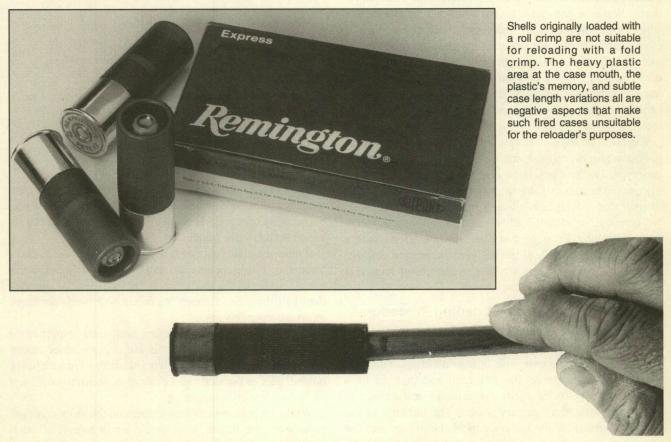
Polyformed cases must always pass the dowel test before reloading.
