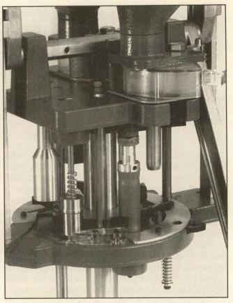
**Caution:** Always check to make sure there is no foreign material in the primer station before placing the primer into the primer tube. If a loose pellet or other material falls into the primer station, the primer could be ignited during seating and present a hazard to the reloader.
