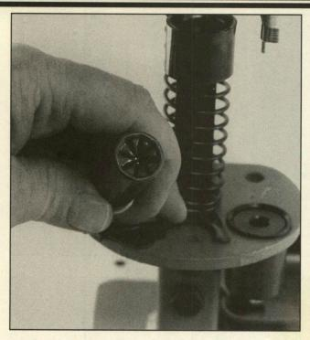
This crimp is the correct depth, but the crimp has failed to close completely. Placing a heavier bevel on the case mouth will often correct this problem. If this does not work, additional wad pressure may be required to leave sufficient case material to form a complete crimp.
