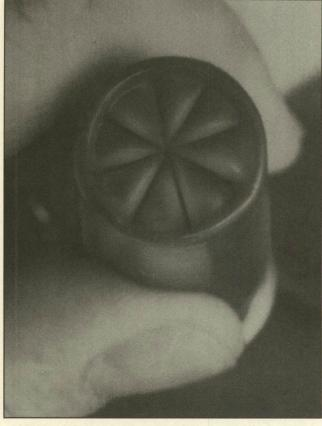
After removing the loaded round from the press, carefully inspect it. Look for a poorly formed crimp, case mouth and body splits, bulges, improperly seated primer or any other reason to reject the shell. If the shell does not pass inspection, correct the problem and/or adjust the loading tool.
