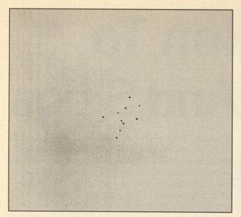
This is a 20-yard pattern, of about 6 inches in diameter, using factory-loaded Winchester buckshot. The reloader will be doing about average if patterns are 2 to 3 times as large at the same range.
