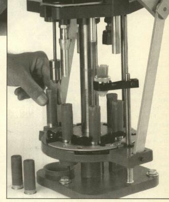
The Apex in the normal sequencee of progressive reloading will have six cases in the shell plate at all times.
