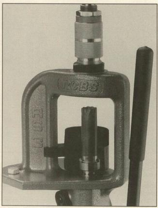
Now, process each case to be reloaded through the sizing/decapping die, placing them in the loading block as they are completed. Unlike metallic cartridge reloading, shotshell cases are not lubricated for sizing. All cases will be processed through each operation before proceeding to the next step.
