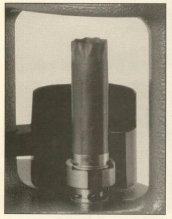
Slip the shellholder into the press ram. Screw the die body into the press and adjust it according to the manufacturer's instructions. The sizing ring and primer decapping rod must be assembled into the die.
