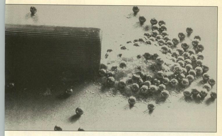
Some premium-grade factory shotshells incorporate a ground polyethylene material as a buffering agent. This material can help prevent some of the otherwise normal pellet deformation and thus produce tighter patterns.
