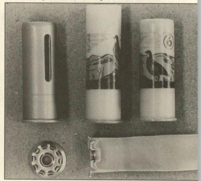
Cases can look different outwardly but be of identical construction internally and hence use identical data. The Activ cases at the extreme left and right are of this nature, having identical construction as shown in the cutaway view. The case in the middle is a new never-loaded component case.
