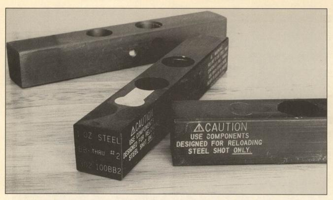
Special shot metering bars are essential for loading steel pellets. Also, such bars are often made to accommodate only specific size pellets. Change pellet size and you may have to change the metering bar.
