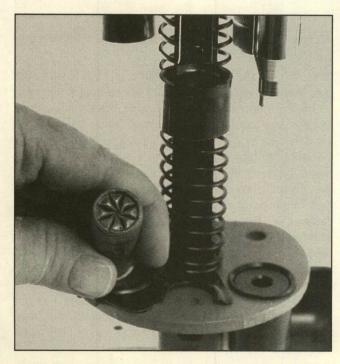
Spiralling is caused by improper tool adjustments or by excess case material in overly stretched cases.
