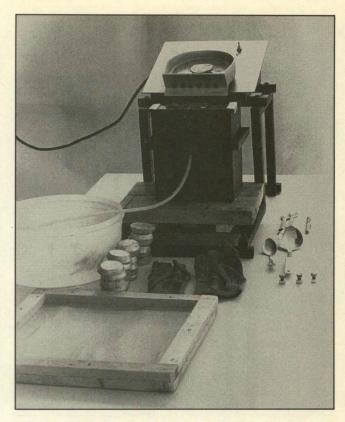
The Littleton shot maker was a unit that enabled the reloader to make acceptable shot for modest applications.
