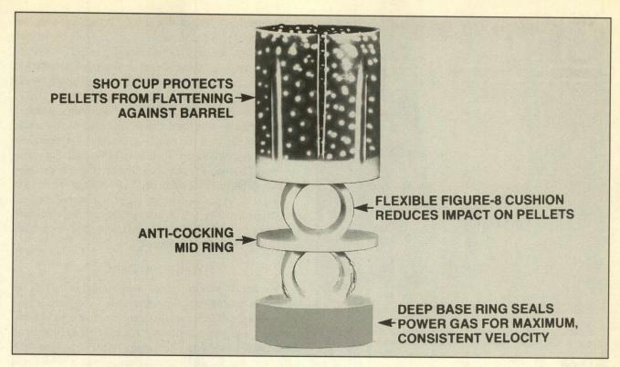
Shotshell wads vary considerably in ballistic performance, but all modern wads have an obturating over-powder cup, a collapsible leg section, and a shot insulating container section.
