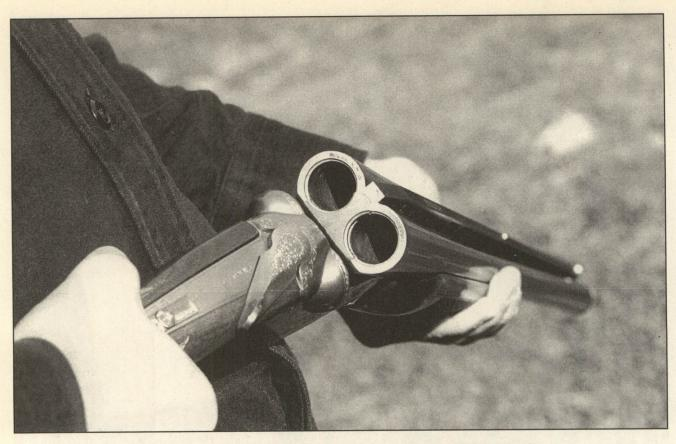
The ammo placed into the chamber will determine the degree of comfort, or discomfort, that the shooter will experience. Free recoil in a 12-gauge gun can range from a comfortable 14 fpe (1-ounce light target loads) to a bone-jarring 51 fpe (17/g-ounce 3-inch magnum loads). The latter has recoil equal to firing 3.6 of the target loads. Fatigue caused by recoil with such loads can quickly exceed a shooter's capability and induce involuntary flinching.
