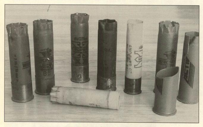
Shotshell cases showing these and any other defects must be culled from cases to be reloaded. When ten percent of the cases in a given lot have been culled, it is time to discard the entire lot. Cases do have finite safe reloading life.
