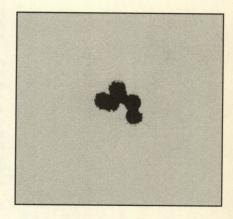
This 50-yard group was fired using a rifled barrel and Winchester slugs.
