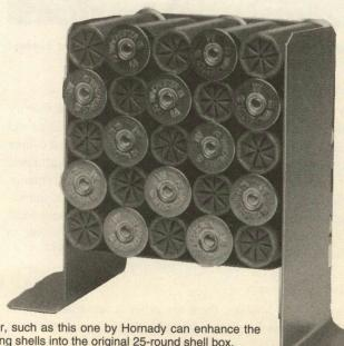
A shell packer, such as this one by Hornady can enhance the speed of getting shells into the original 25-round shell box.
