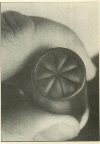
Remove the loaded round from the reloading tool and carefully inspect it. Look for poorly formed crimps, case mouth and body splits, bulges, improperly seated primers or any other reason to reject the shell. **Caution:** Do not use any ammunition that does not pass your visual inspection. Discard all such ammunition is a safe manner.
