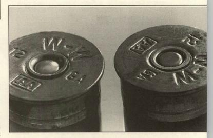
Primers must be seated so as to make the battery cup flush with the case head. The primer on the left is too high and the loaded round should not be used. The primer on the right is correctly seated. A small gap between the primer battery cup and case head, as shown on the right shell, can be normal.
