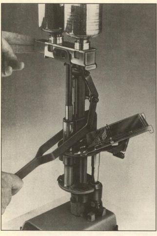
With the press handle held down, move the shot charge bar from left to right with the left hand. This will drop the shot into the case. Now raise the press handle.
